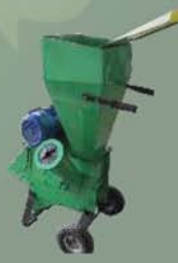
Agri Waste Chipper Machine Capacity = 300 kg per hour
