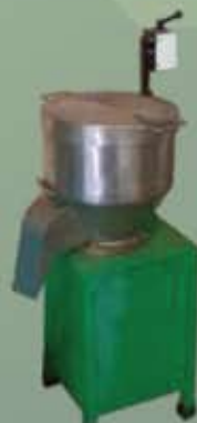
Food Waste Crusher Capacity = 150-200 kg/hr.
